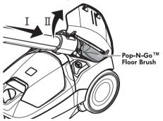
**NOTE:** If there is difficulty attaching brush to wand in the manner described above, simply remove the brush from storage compartment and insert it into the wand collar.
