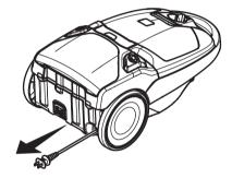
**2.** Plug the polarized power cord into a 120 Volt outlet located near the floor.
