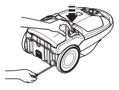
3. Lower wand from upright position by pressing on the HANDLE RELEASE pedal.
