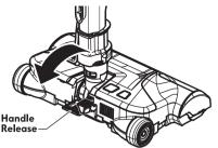
**4.** Select a pile height setting by pressing the height adjust pedal on the rear of the PowerMate<sup>®</sup>. The pile height setting shows on the indicator.
