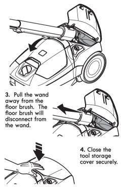
**NOTE:** If there is difficulty detaching the wand from brush in the manner described above, simply press the Tool Release button to disconnect brush from wand.
